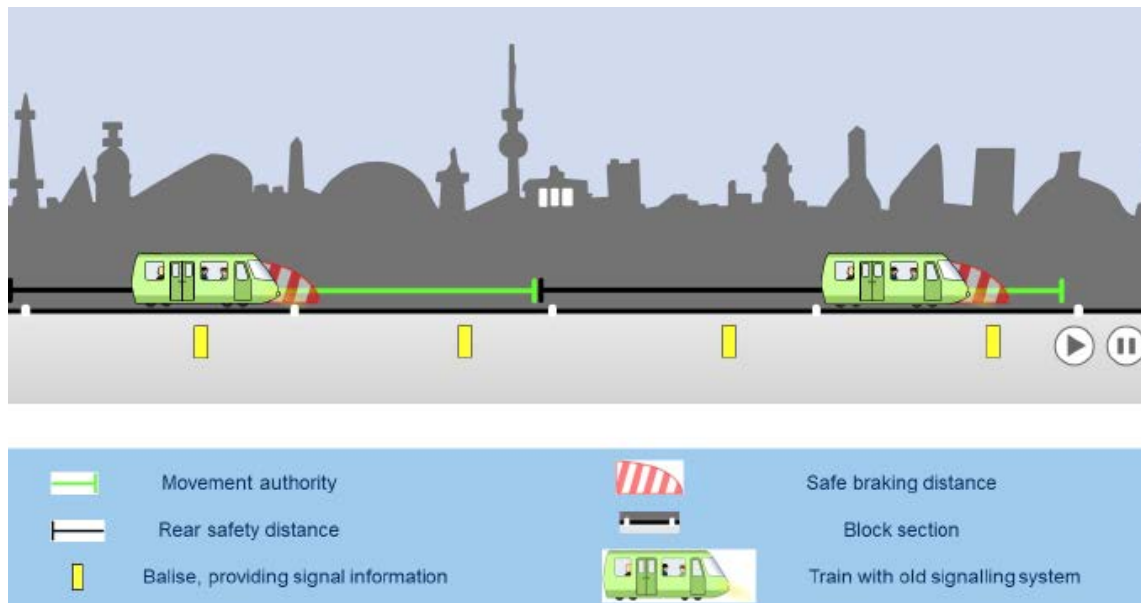
Figure 14: Urban signalling (Metro) – Conventional technology
