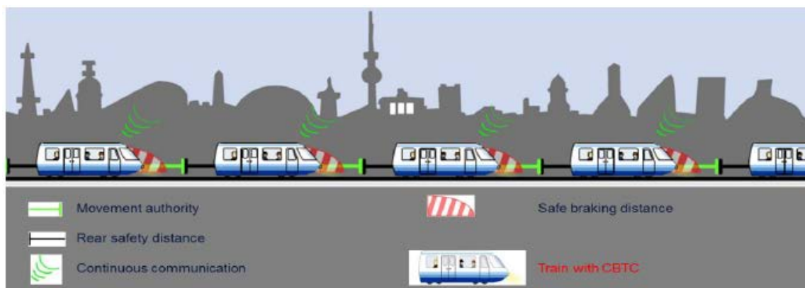
Figure 15: Urban signalling (Metro) – CBTC technology
